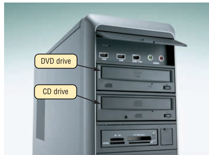
FIGURE 4-25 External drive bays usually are located beside or on top of one another.
