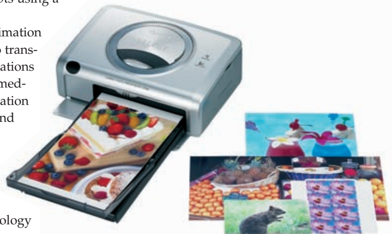
FIGURE 5-39 The printer shown in this figure uses dye-sublimation technology to create photographic-quality output for the home or small office user.
