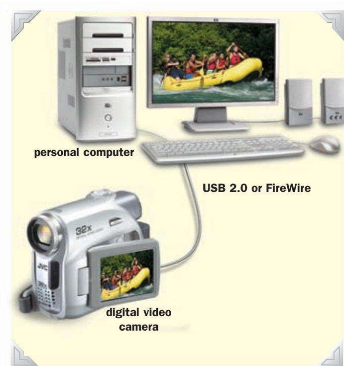
FIGURE 11 A digital video camera is connected to the personal computer via a FireWire or USB 2.0 port. No additional hardware is needed.
