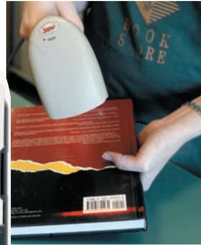
FIGURE 5-21 A bar code reader uses laser beams to read bar codes on products such as ID cards and books.
