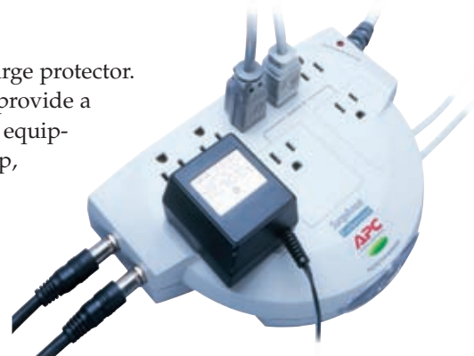
FIGURE 10-13 Circuits inside a surge protector safeguard against overvoltages and undervoltages.
