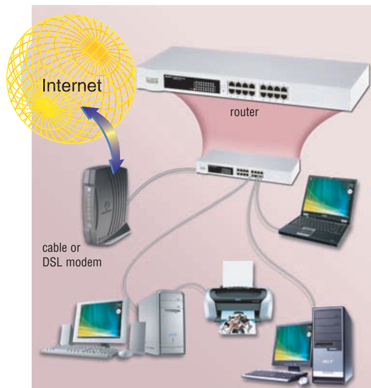
FIGURE 8-21 Through a router, home and small business networks can share access to a high-speed Internet connection such as through a cable or DSL modem.
