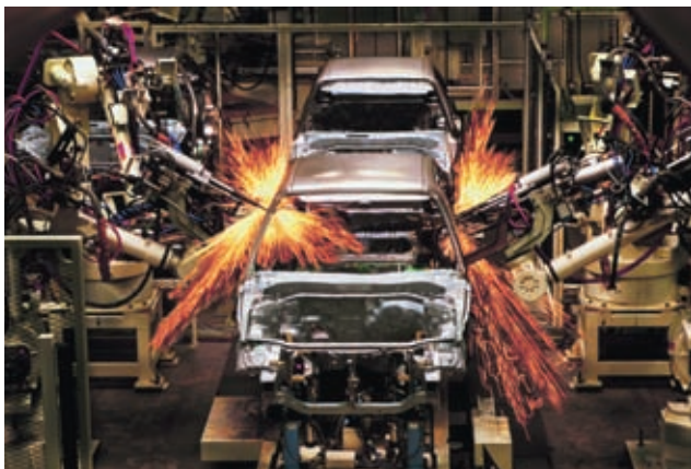
FIGURE 1-37 Automotive factories use industrial robots to weld car bodies.
