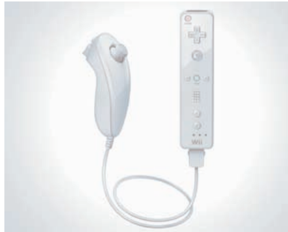
FIGURE 15 Nintendo's Wii gives gamers new experiences with motion control. The Wii comes with several input devices; the Wii Remote and the Nunchuk use a device called an accelerometer, which measures acceleration forces electromechanically. The accelerometers sense motion and transmit a signal using Bluetooth technology to a sensor bar, which can be up to 30 feet away. Up to four Wii Remotes can be connected simultaneously for multiplayer interaction.
