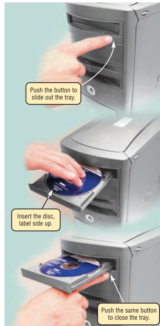
FIGURE 6-14 On optical disc drives, you push a button to slide out a tray, insert the disc with the label side up, and then push the same button to close the tray.
