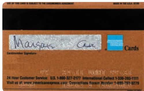
FIGURE 5-23 A magnetic stripe card reader reads information encoded on the stripe on the back of your credit card.
