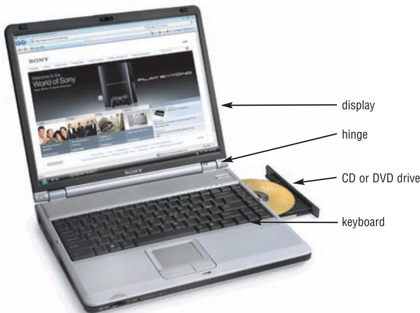
FIGURE 1-15 On a typical notebook computer, the keyboard is on top of the system unit, and the display attaches to the system unit with hinges.
