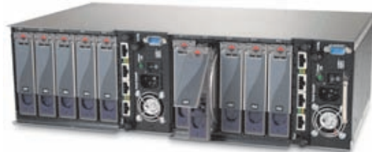
FIGURE 12-22 A group of two or more integrated hard disks, called a RAID (redundant array of independent disks), often is used with network servers. Shown here is a rack-mounted RAID chassis including the hard disks.
