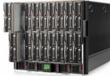
FIGURE 12-25 A blade server contains several very small servers, each on its own blade within the server.
